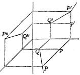
by D. The line D will be the hypothenuse of a triangle, of which the base is QP, and altitude p'P'.
